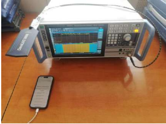
Figure 1: Measurement set-up showing the receiving omnidirectional antenna connected to the signal analyzer and the Iphone 14 Pro phone
