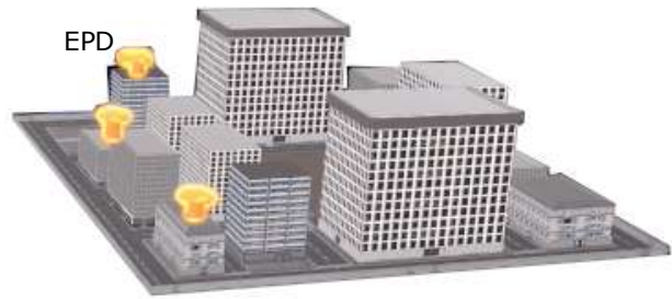
Figure 3: A pictorial view of an EPD; it consists of an array of electromagnetic controllable scattering elements optimized to maximize the capacity of the wireless system. The DPL contains all the resources regarding space/time/polarization degrees of freedom of the electromagnetic field that the communication system can use to encode information while EPDs allow the maximization of these resources by increasing the number of possible distinguishable field configurations by the receiver, acting as 'lenses' for physical information.
